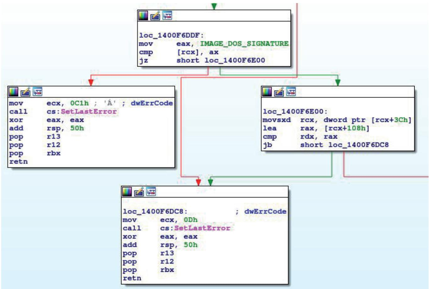
Figure 4: Code from the MemoryModule memory injection library.
